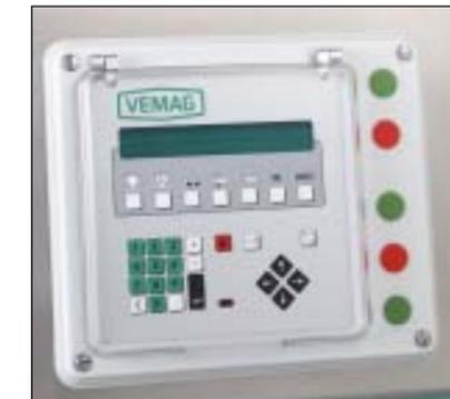
to 99 programs under their names. Settings are entered using the digital keypad of the portioning computer and confirmed with a single key. Weight corrections can be entered directly in grammes. All output is shown in clear text in the desired language. A protective cover protects the portioning computer from splashes.
