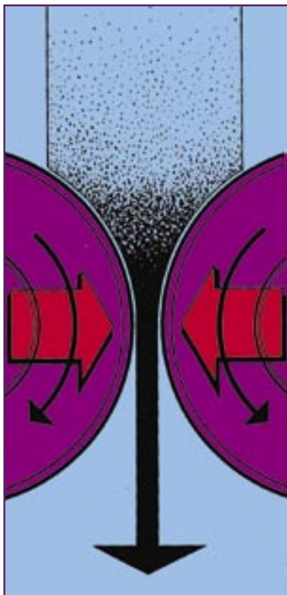
Fig. 1 BASIC CONCEPT OF ROLL PRESSING
