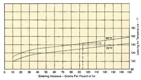
LEAVING AIR TEMPERATURE . 1F FOR INLET TEMPERATURE BELOW 75°F, SUBTRACT TEMPERATURE DIFFERENCE FROM OUTLET TEMPERATURE
