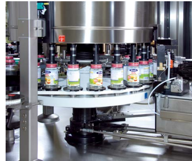
Containers turned by container plates with servomotors (photograph on the left)
