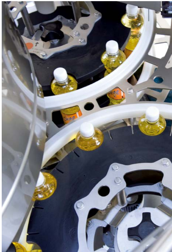
Raptec guidance handling parts with PET bottles
