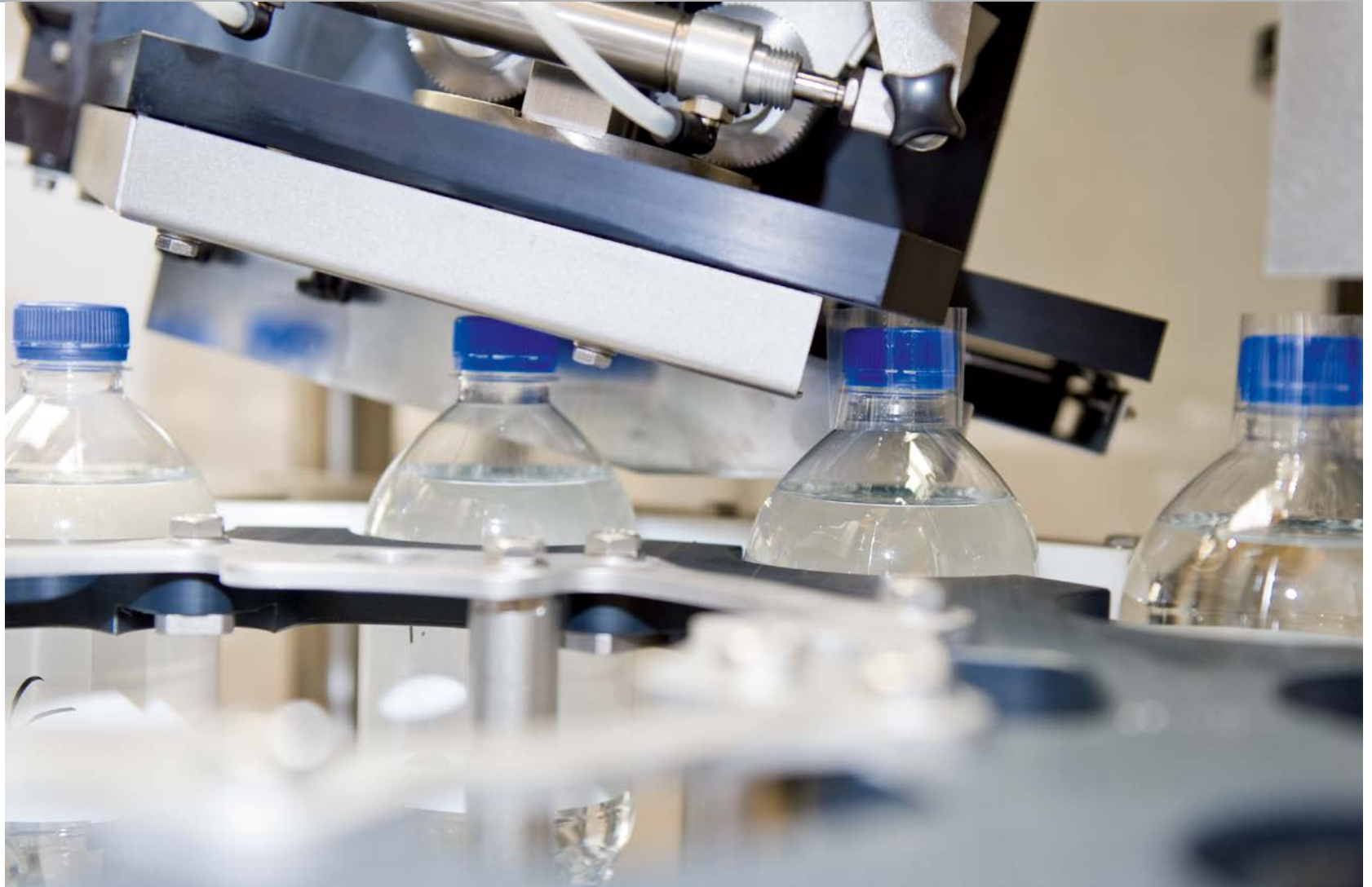
KRONES Garantomat for attaching a shrink sleeve as the tamper-evident seal
