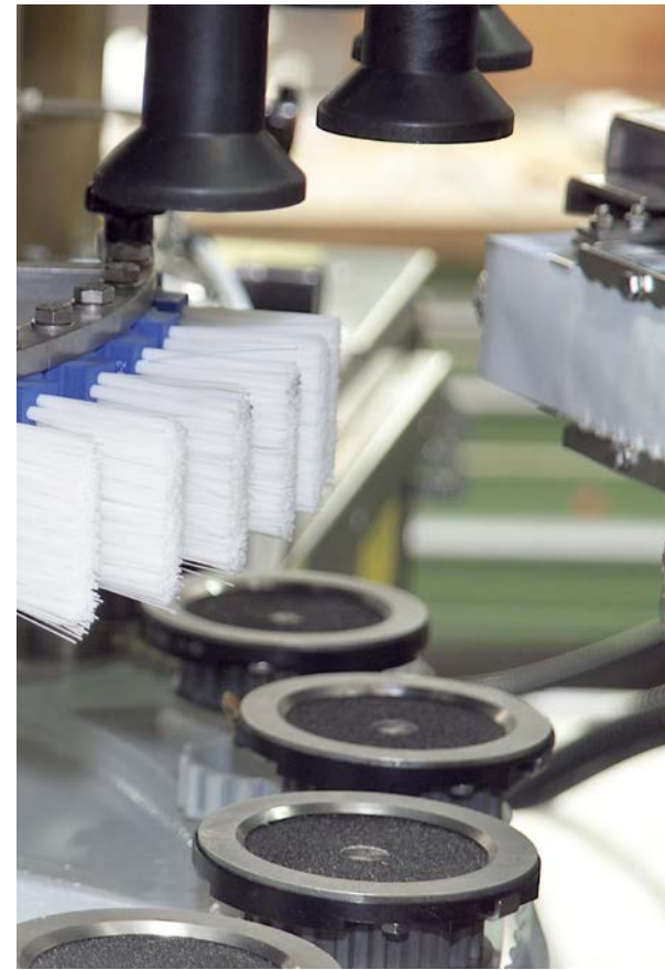
Container plates and brushing-on station designed for quick changing
