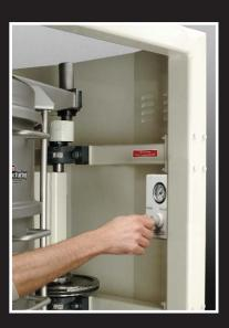
Our horizontal gyratory motion is gentle. It reduces product degradation and is superior to designs using vibratory or centrifugal action.
