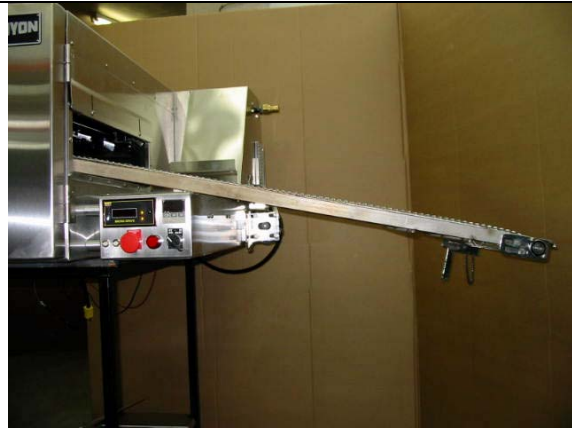
10. Remove conveyor completely.
