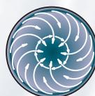
90 Lead – Keeps oversize material from being discharged and assists in receiving maximum throughput of minus material which tends to “ball”
