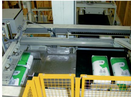
Layer formation on the PLS palletizer. To the right bags on the infeed belt, to the left ready bag layer on the slide plate
