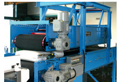
Bag flattening station
