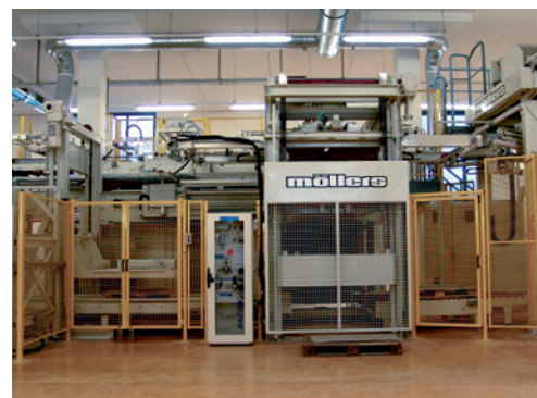
Corrosion-protected PLS-C palletizer in a packaging line for evaporated salt
