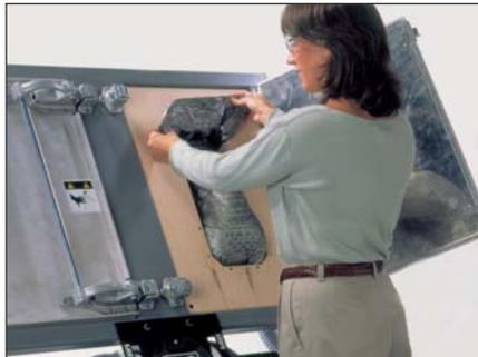
When placed into the vertical mold enclosure, the foam-filled bag is drawn into the mold by an on-board vacuum.
