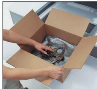
The product is placed onto the foam-filled bag as it expands in the carton, forming a custom-fit cushion.
