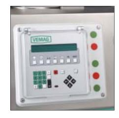
work. The control panel with integrated 10-key keypad was ergonomically designed. Up to 99 programs and their names can be stored. The operator enters set values using the 10-key keypad of the portioning computer and confirms them with a single key. Weight corrections can be entered directly in grammes. All output information is shown in clear text in the desired language. A protective cover keeps splashes off the portioning computer.
