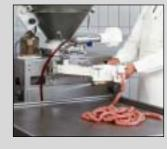
Length portioning device LPV 802 for linking sausages in natural casings with identical lengths, identical weights and identical calibres
