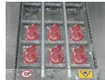
Loading zone Products are loaded into formed pockets
