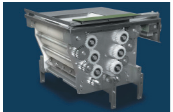
Dough capacity: approx. 17,23 or 28 litres for 4-, 5- or 6-row execution of the REX
