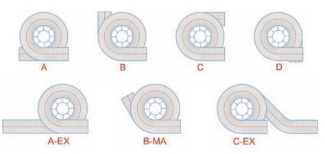
The position of the in feed tangent on up spirals and out feed tangent on down spirals can be customized to meet specific layout requirements. Samples are shown above (A-EX, B-MA and C-EX). A horizontal section is provided at in and out feed to assure smooth transition between conveyors. All Ryson Spirals are available in powder coated carbon steel, stainless steel, washdown, and freezer versions.
