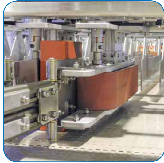
Side Power Diverter
