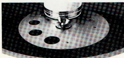
Unique, externally controlled feed orifice valve permits flow adjustments without emptying the bin.
