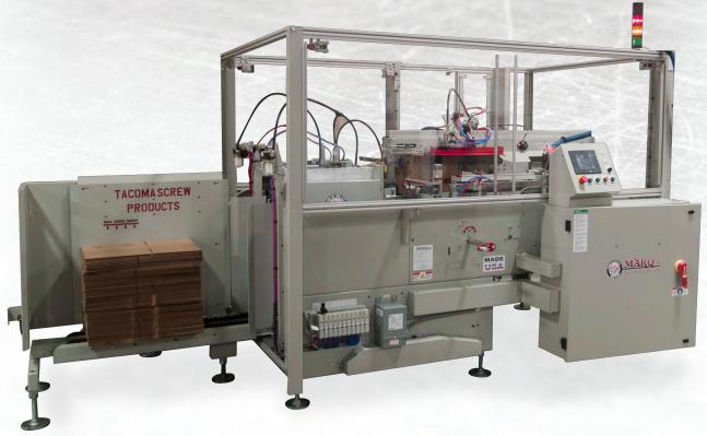
MARQ Packaging's Case Erector Bottom Sealer with Bundle Hopper is a design that features added versatility while maintaining the high standard of quality and performance expected in a MARQ machine. Its superior style of bundle hopper is easily accessible for adjustments and servicing and reduces the amount of lifting required by the operator.
