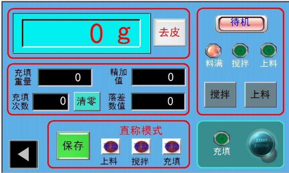
C.2.1 Pure bonus: when the actual filling weight reaches the set value, filling screw speed, the highest speed drop is starting speed。
