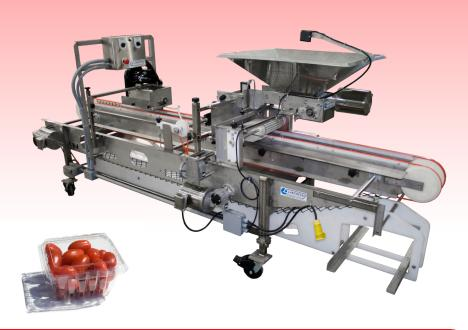
**Features:** Quick Changeover (Adjustable from 4.4 oz to 2.75lb - no tools necessary) // Easy Maintenance (Filler is built with an easy-to-clean, open design) // Includes powered 'paddle-closer' // Adjustable hopper height from 42" to 52" to fit in almost any existing line
