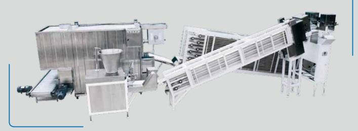
The Compact Line is the smallest Automatic Line to produce the Lebanese / Pita Bread. It is economical and does not require large spaces for operation. This device is efficient and is mostly adopted for hypermarkets, big restaurants and small retail bakeries. Moreover, the Compact Line can be manufactured in metal steel chassis covered with appropriate colouring or in full stainless steel with distinct touching for direct display of the merchandise.
