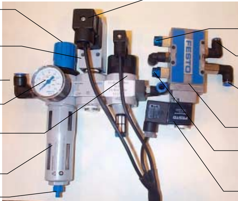
Figure 8.11 Pusher and Plough Reject Components
