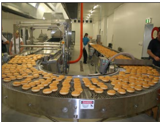
Above: Century system with 180° curve conveyor
