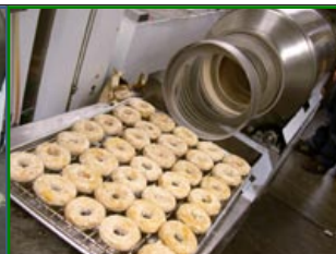
Discharge onto screen
