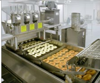
MODEL C6-24 — 6 ft. fryer, 6 standard donuts per pocket, shown at right with MDDRF-6 cake donut depositor. C6-24 is a gas-only fryer.
