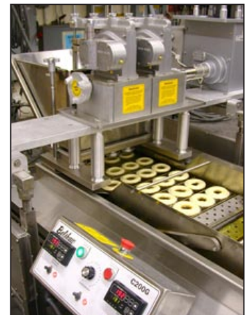
Right: Multimatic MDDRF-4 deposits 4 donuts across the fryer, shown with C6-16G fryer
