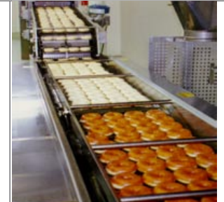
MODEL C10-16 — 6 ft. long fryer, 4 standard donuts per pocket, frying raised donuts (right). Gas and electric models available.
