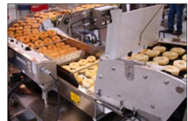
Below: Century - Mark VI system in operation. Frying and proofing functions are synchronized.
