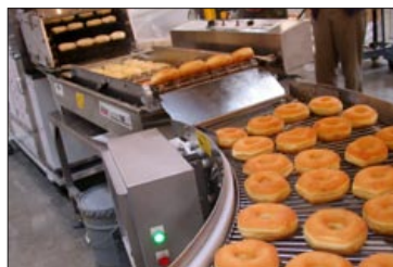
Below: Century - Mark VI system in operation. Frying and proofing functions are synchronized.
