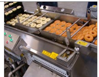
MODEL C6-16 — 6 ft. long fryer, 4 standard donuts per pocket, frying raised donuts (right). Gas and electric models available.
