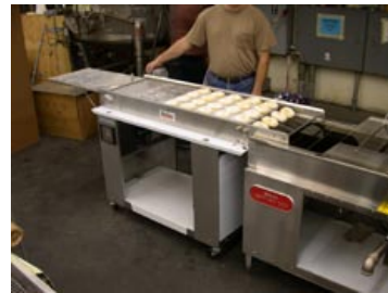
FT200 Feed Table with one cloth of donuts. (The Feed Table can hold 2 cloths with donuts)
