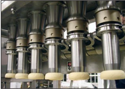
◀ Belshaw Pressure Cutter producing Ring donuts
