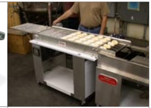
Feed table in operation
