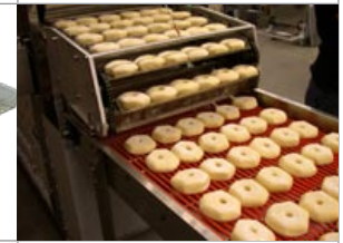
Transfer conveyor in operation
