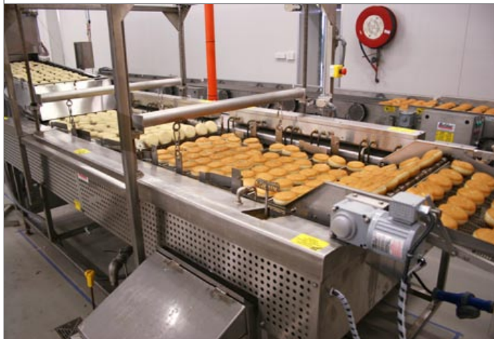
MODEL C10-24 — 10 ft. fryer, 6 standard donuts per pocket, part of a donut system frying raised donuts. Gas and electric models available.
