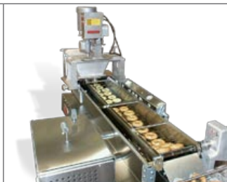
MODEL C6-8 — 6 ft. fryer, 2 standard donuts per pocket, shown with MD-2 cake donut depositor. C6-8 is electric only.
