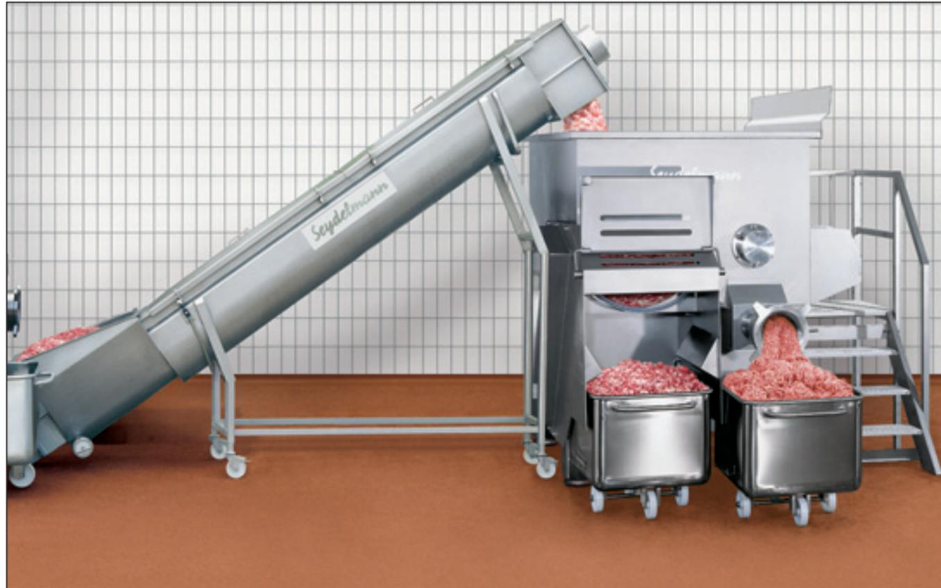
Mixer-Grinder PG 160 with movable screw conveyor
