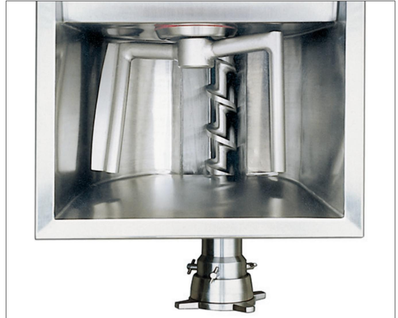
Mixing and automatic feeding - on request with forward and reverse drive
