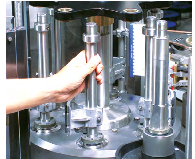
KRONES cold-glue labelling station (left picture)
