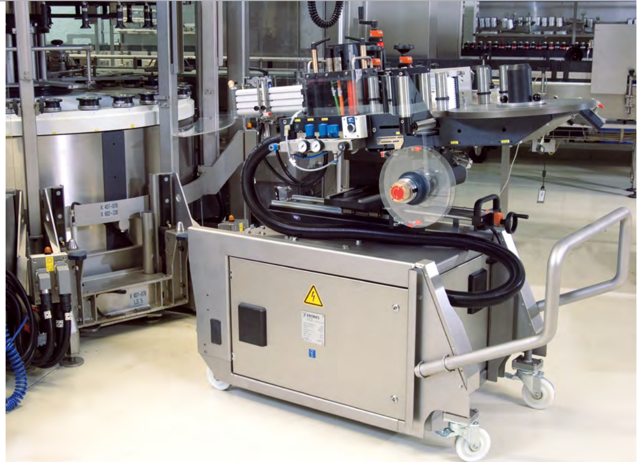
Changing a labelling station
