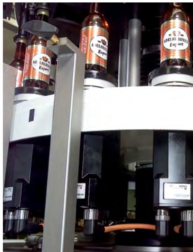
Container table with servomotors, protection type IP65
