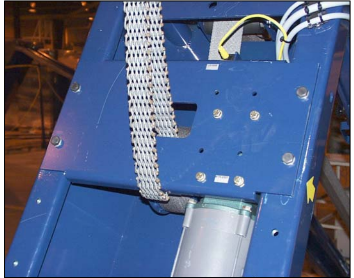
Wrap Arm Balance Point - Mounting The Wrap Arm
