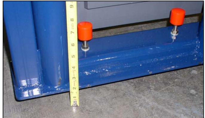
Measurement Between Wrap Arm And Floor
