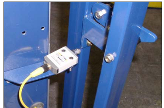
Safety Bumper Switch – Bumper Extended
