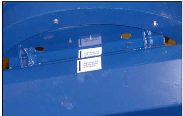
Wrap Arm Mounting And Alignment
