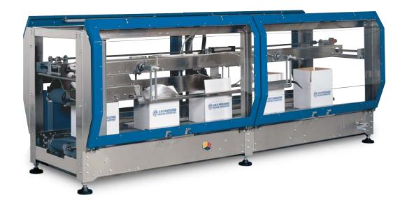
Small in size, but a giant in production, the Model 336 is built strong and tough to tackle the most demanding case sealing challenges you face today. Whether linked to a drop packer or feeding cases from one or multiple lines, the 336 provides reliable, continuous operation. Send cases spaced or back to
