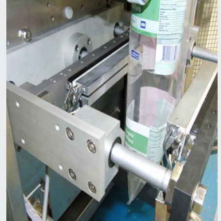
Chainless jaw assembly gives you higher sealing force, improved hygiene and reduced maintenance
