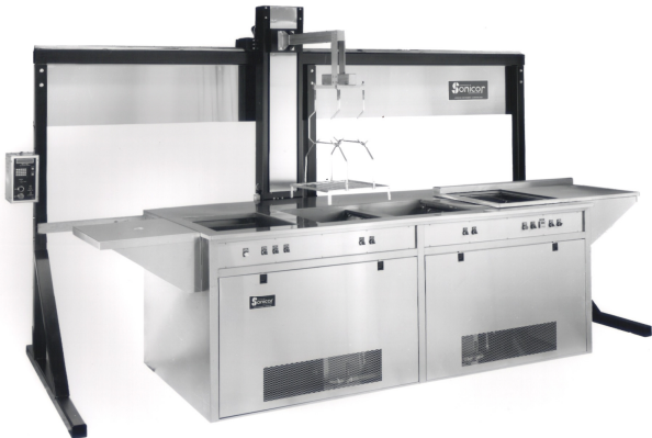
CPS4-1620 with RCT-50 automation process control system
