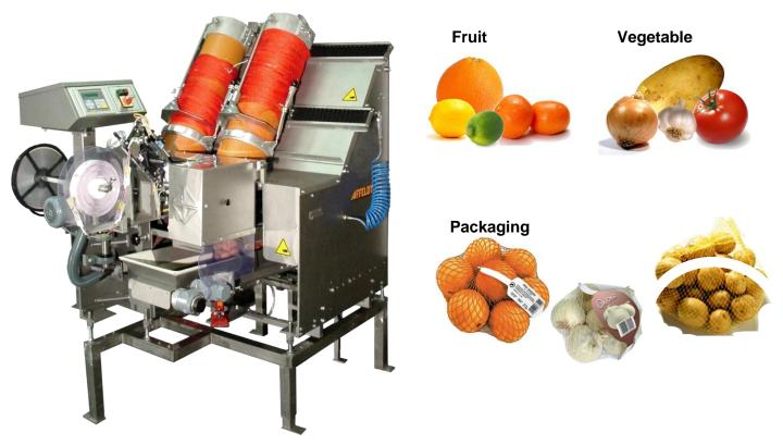
The net clipping machine AVN 929 packs solid goods such as citrus fruits, potatoes, onions, garlic, tomatoes and similar products, which have been previously accumulated by a weighing or counting machine, speedily and efficiently into nets. The large scope of equipment allows for the clipping machine to be adapted to a wide range of products.
