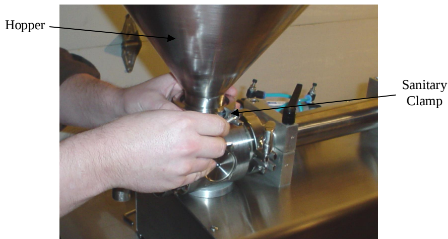
Figure 5-1 Hopper Tank Removal
