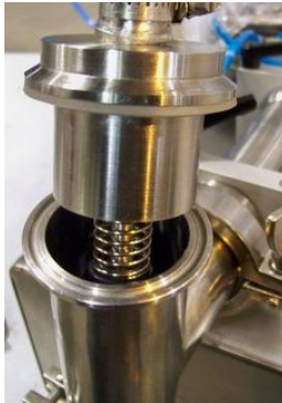
Figure 5-10 Fill Check Valve
