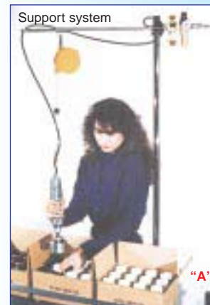
Electronic Machine Torque Monitor shown on Kaps-All's Automatic Cap Tightener
