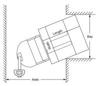
Aisle dimensions listed above assume 4" between loads. Use the larger dimension; load width or load length. For ease of use and add 6" to 12" for operator clearance to the appropriate specifications listed above. Truck performance may vary due to application requirements' and changes in model design.
