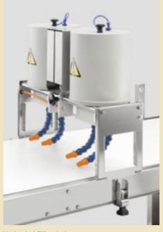
Mechanical filling device For creamy to semi-viscous, self-flowing fillings, the Polyline can also be equipped with a mechanical filling device
