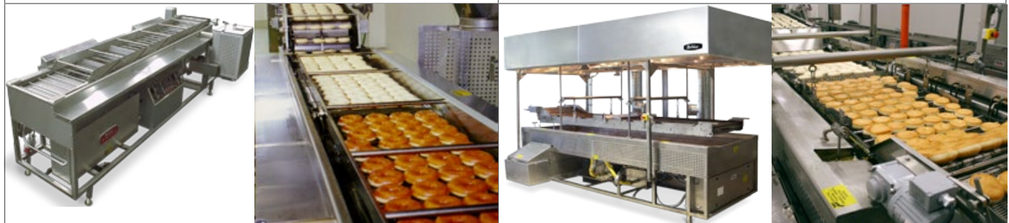
Century C10-16 — 10 ft. fryer, 4 standard donuts per pocket, shown at right with TM400 automatic proofer. Gas and electric models available.
