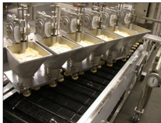
Above; Belshaw Vacumatic – deposits ring donuts directly to automatic proofer
