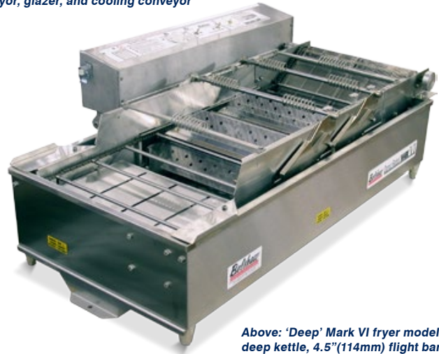
Above: Century – Mark VI system with proofer, Mark VI 'Deep' fryer, 180° curve conveyor, glazer, and cooling conveyor
