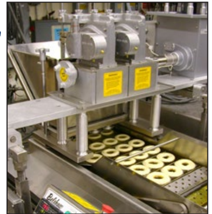
Multimatic MDDRF-4 deposits 4 donuts across the fryer, shown with C6-16G fryer
