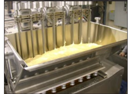
Multimatic MS-6/8/9/12 deposits 8 donuts at a time, compatible with C6-24 / C10-24 and C14-24 fryers
