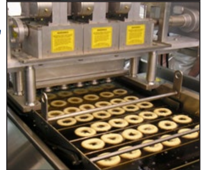
Multimatic MDDRF-6 deposits 6 donuts across the fryer, shown with C6-24G fryer
