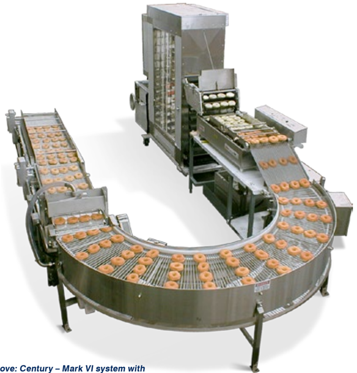
Above: Century – Mark VI system with proofer, Mark VI 'Deep' fryer, 180° curve conveyor, glazer, and cooling conveyor
