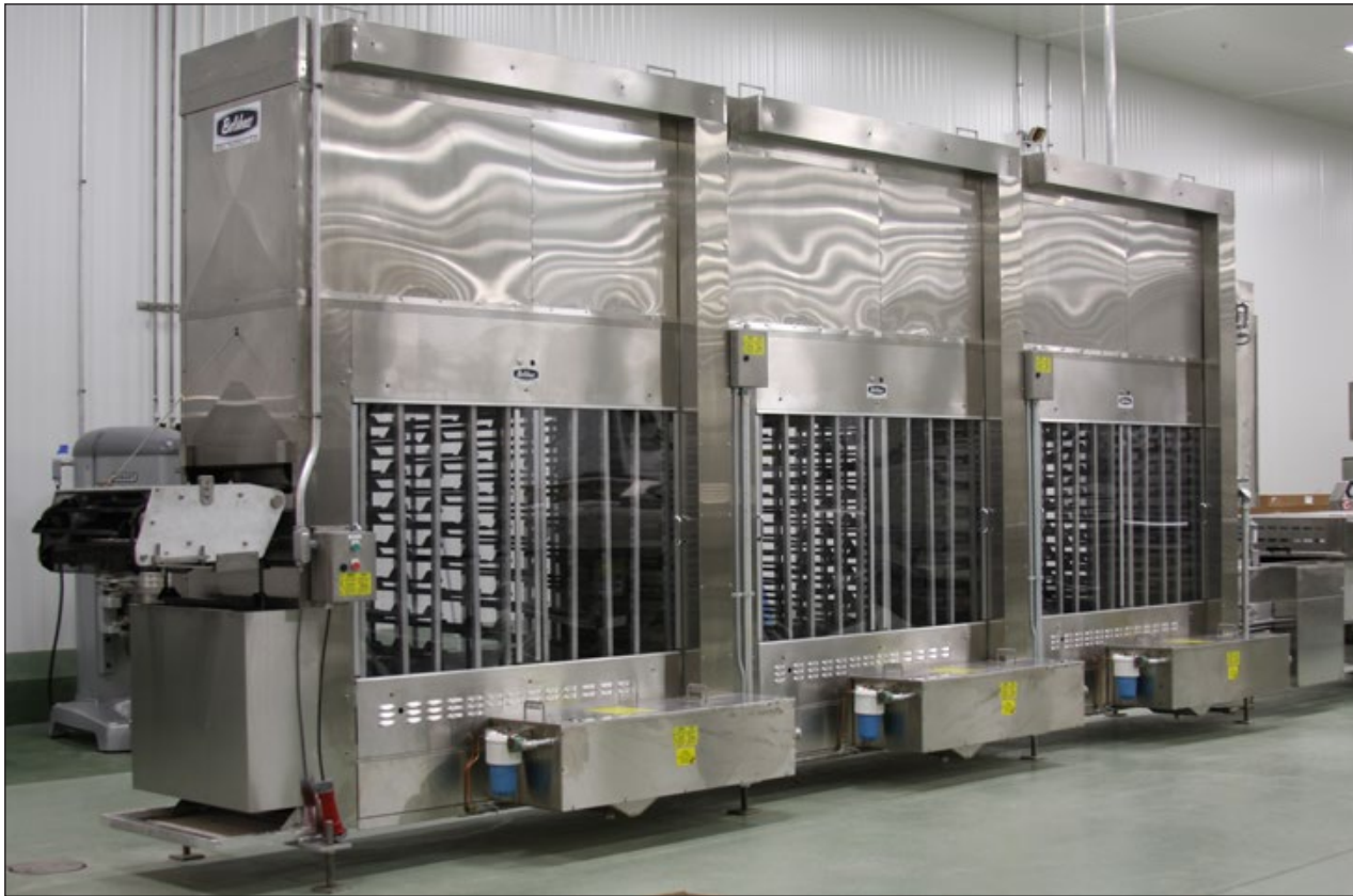
Above: TM600 3-section proofer – compatible with C10-24 fryers
