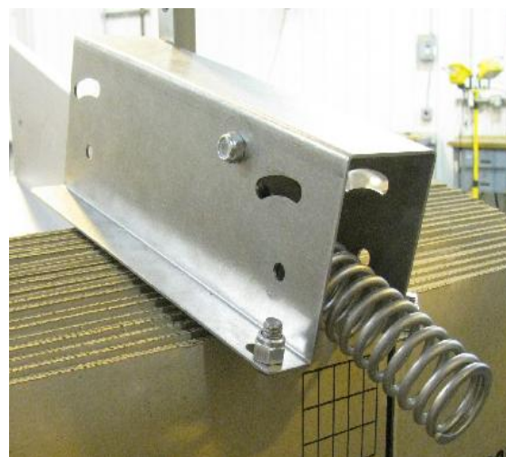
Figure 18 Case Opener Spring (viewed from inside of machine)
