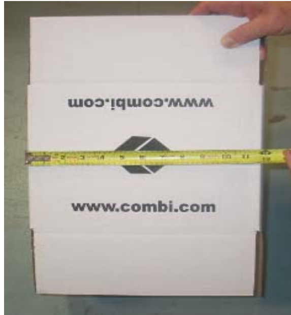
Figure 11 – Measuring Major Panel (Case Length)
