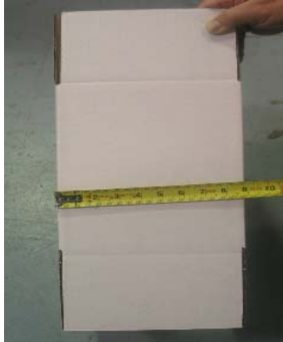
Figure 4 – Measuring Minor Panel (Case Width)
