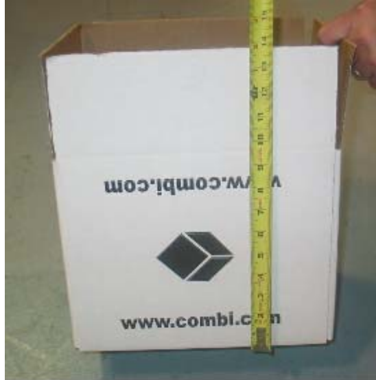
Figure 13 – Measure Case Height (RSC case type)
