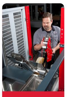
The CE-10's hinged case hold down plate allows for easy tape head removal. The case erector's open design without overhead cross members provides easy access for planned maintenance.
