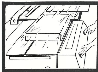
After product is transferred to sealing area, operator presses palm buttons to activate sealing head.
