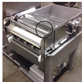
Rotary filter Can be optionally equipped with a scraper, chute or self-cleaning.
