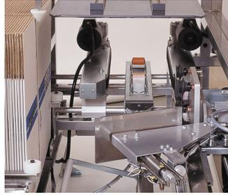
Efficient flap folding and closing system.
