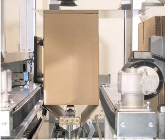
Efficient bottom flap folding and glue application.
