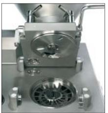
residues thus eliminating bacteria build-up. The machines can guickly and easily be cleaned using low-pressure equipment. As there are no lockable compartments or closed steps, all surfaces dry very quickly after cleaning.
