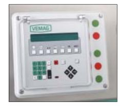
to 99 programs under their names. Settings are entered using the digital keypad of the portioning computer and confirmed with a single key. Weight corrections can be entered directly in grammes. All output is shown in clear text in the desired language. A protective cover protects the portioning computer from
