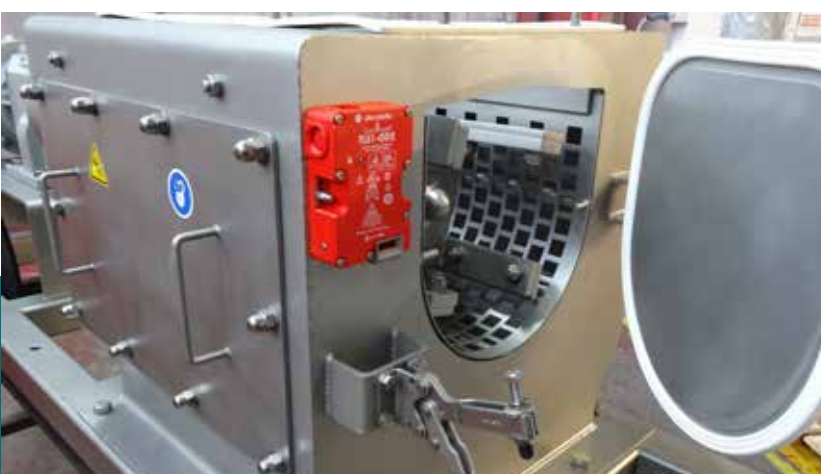
View of Cantilever Shaft and Hinged End Door
