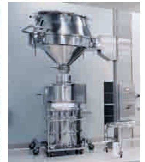
An inverted fluid-bed dryer bowl directly discharges into a Comil® U30 on a portable stand, feeding a stainless steel drum.
