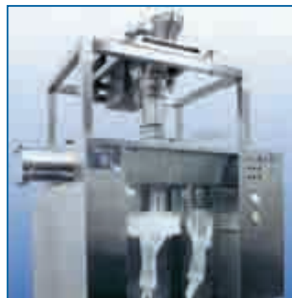
Quadro custom engineered this integrated milling solution incorporating the Comil® with a Carlisle Extract crossflow system.
