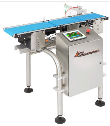
The Model EW-8 is All-Fill's economical solution for users and applications that may only require an entry level checkweigher. The EW-8 offers 0.5g resolution. It utilizes a strain gauge load cell for weighing packages up to 5 lbs and operating at speeds up to 120 packages per minute, this makes the EW-8 just as versatile and reliable as other All-Fill models.
