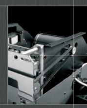
Powered Unwind, exclusive to Autobag systems, provides web alignment and tension control for consistent film delivery to product load station.
