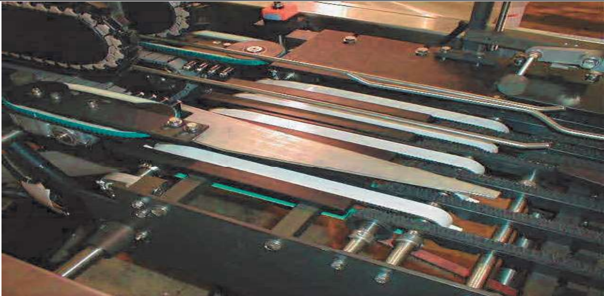
Figure 2. View of turn correction and transfer section
