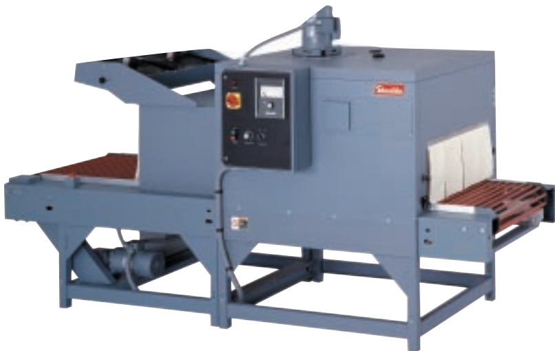
Shanklin Poly Shrink Tunnels feature an annealing chamber following the shrinking chamber and a cooling fan to allow the polyethylene film to set prior to handling.
