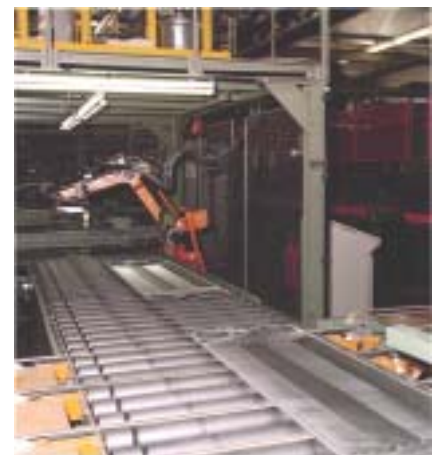
Robot controlled gasket gluing assembly
