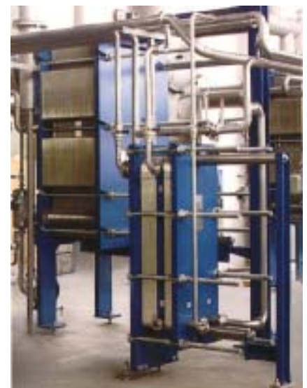
SIGMASTAR® evaporator and SIGMA plate heat exchanger
